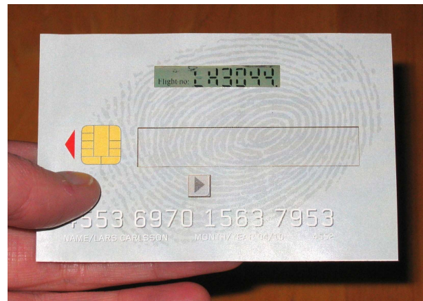
Figure 6. Reflective flexible TN-LCD with SD-1/SDA-2 alignment layer mounted in smart card prototype.
