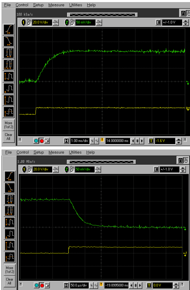
Figure 7: Switching response time of NBB cell. Top: Off time; Bottom: On time.
