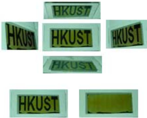
Figure 4. Bistable pattern shows permanent bistability and excellent viewing angles.
