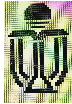
Figure 7. The image generated by 7 \mu\text{m} 64 \times 64 passively addressed photo-aligned FLC display, which is memorized after the driving voltage is switched off.
