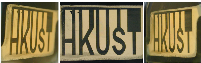
Figure 6. 1.5 \mu\text{m} photo-aligned FLC-497 display with good bistability and wide viewing angle after the driving voltage was switched off.
