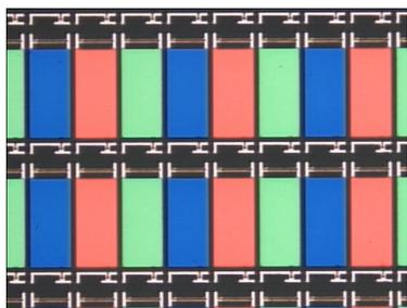
Figure 8. Photograph of magnified RGB pixels.
