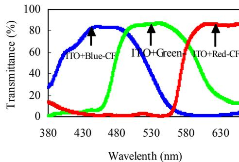
**Figure 7. Optical transmissions of CFs covered by the room temperature ITO.**
