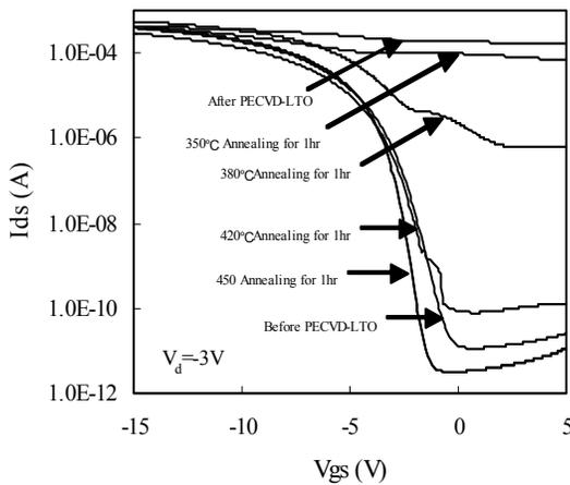
**Figure 5. Transfer characteristics of MILC poly-Si TFT before and after the formation of PECVD SiON (The characteristics after nitrogen and forming gas annealing are also shown.)**
