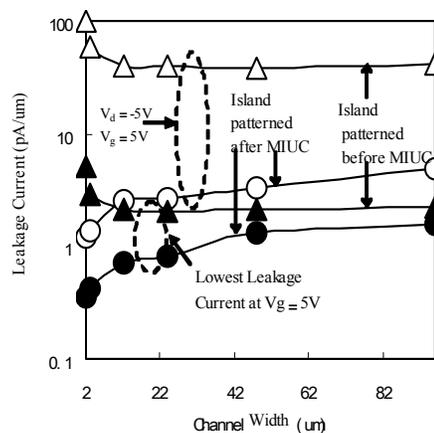
**Figure 4. Dependence of the leakage current per unit channel width on the channel width of Types A and B TFTs.**
