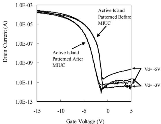
**Figure 3. Transfer characteristics of p-type MILC poly-Si TFTs with active islands patterned before and after MILC at different drain bias voltage  $V_d$ .**
