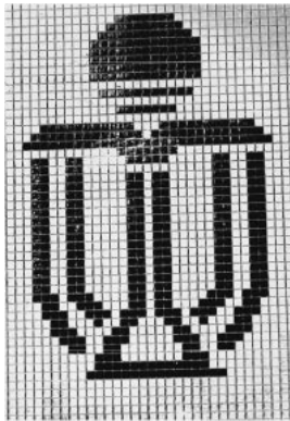
Fig. 16. Image generated by a passively addressed photo-aligned 64 \times 64 FLC display, which is memorized after the driving voltage is switched off. The FLC-408A layer thickness is 5\ \mu\text{m} .
