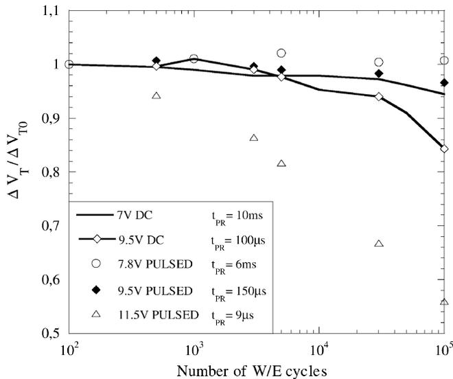
Fig. 4. Relative variation of the program window during cycling measured using a dc bias (solid line) and the pulsed tunnel technique (symbols) with three different waveforms.
