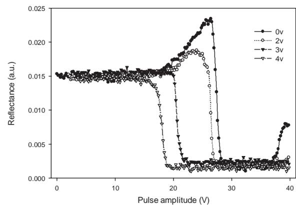
Fig. 2. Reflectance against pulse amplitude at different signal floor voltages. The frequency of both bipolar pulse and signal floor voltage is 250 Hz, whereas the writing time is 4 ms.
