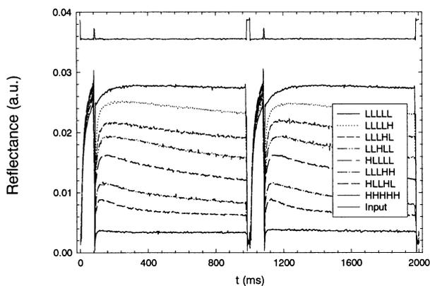
Fig. 3. Dynamic response of gray-scale control. The writing time is 5 ms and the clearing time is 20 ms. Both have the same frequency at 1 kHz. The high H, low L and data voltages are respectively 0.58, 0.3 and 0.14. The drive voltage is 36.4 V peak. The vertical axis represents the intensity and it has an arbitrary unit.
