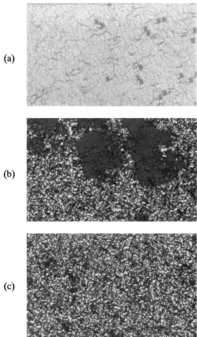
Fig. 4. Photographs of different topological domains: (a) planar, (b) coexistence of planar and focal-conic, (c) focal-conic. The magnification is 50 and the grey round dots are the spacers.
