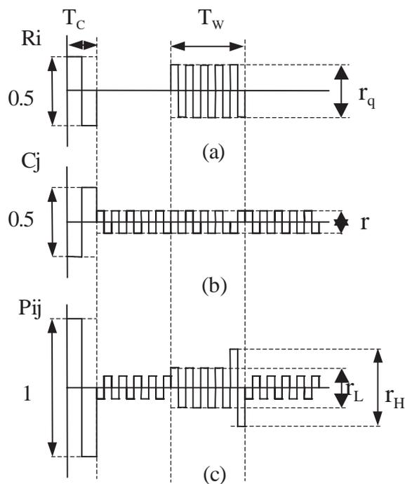
Fig. 1. Waveforms of pulse sequence to address the gray-scale BCD.
