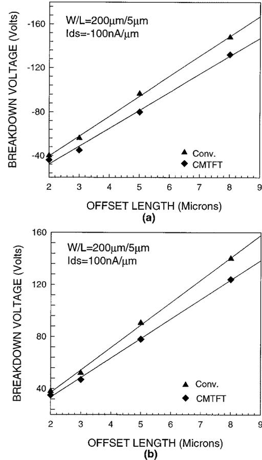
Fig. 7. Breakdown voltage versus offset length of the (a) p-channel poly-Si/Si<sub>1-x</sub>Ge<sub>x</sub>/Si CMTFT and (b) n-channel poly-Si/Si<sub>1-x</sub>Ge<sub>x</sub>/Si CMTFT.
