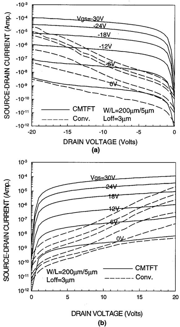
Fig. 4. Forward conduction characteristics of the (a) p-channel poly-Si/Si<sub>1-x</sub>Ge<sub>x</sub>/Si CMTFT and conventional offset drain TFT, and (b) n-channel poly-Si/Si<sub>1-x</sub>Ge<sub>x</sub>/Si CMTFT and conventional offset drain TFT.
