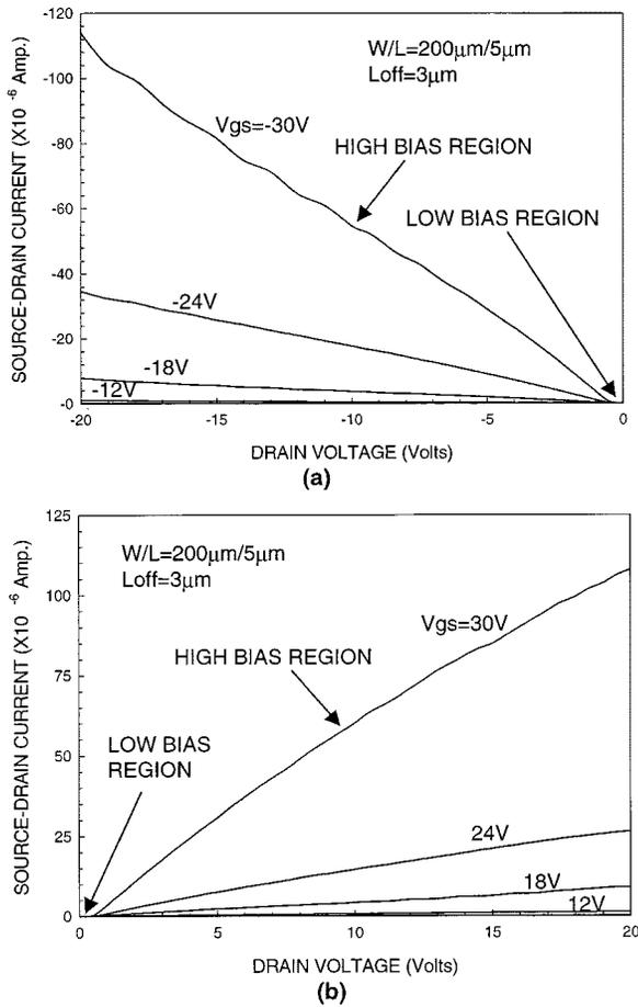
Fig. 3.  $I$ - $V$  characteristics of the (a) p-channel poly-Si/Si<sub>1-x</sub>Ge<sub>x</sub>/Si CMTFT, and (b) n-channel poly-Si/Si<sub>1-x</sub>Ge<sub>x</sub>/Si CMTFT.
