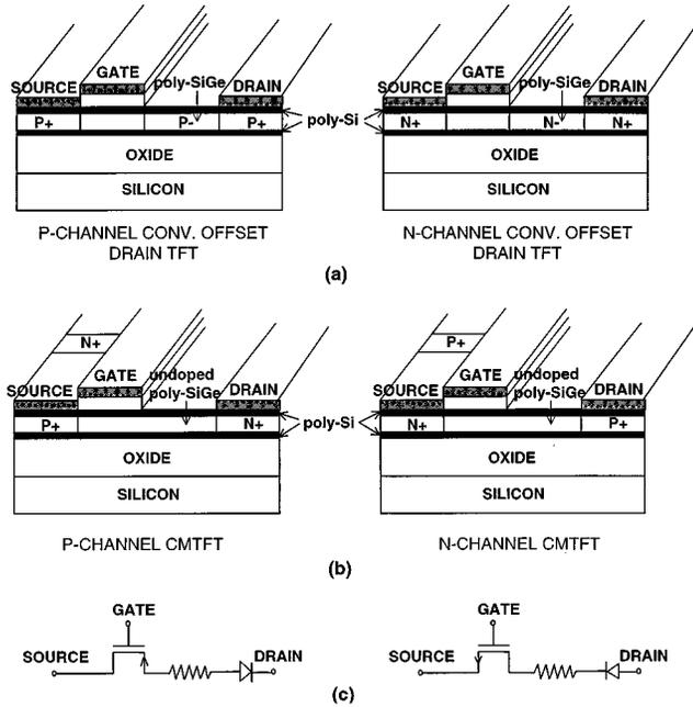
Fig. 1. Schematic cross section of the p- and n-channel poly-Si/Si<sub>1-x</sub>Ge<sub>x</sub>/Si (a) conventional offset drain TFTs, (b) CMTFTs, and (c) the equivalent circuit model for Fig. 1(b).
