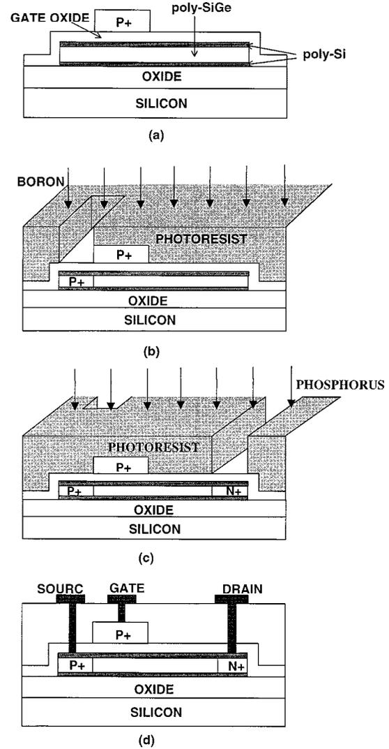
Fig. 2. Major fabrication steps of the p-channel poly-Si/Si<sub>1-x</sub>Ge<sub>x</sub>/Si CMTFT.
