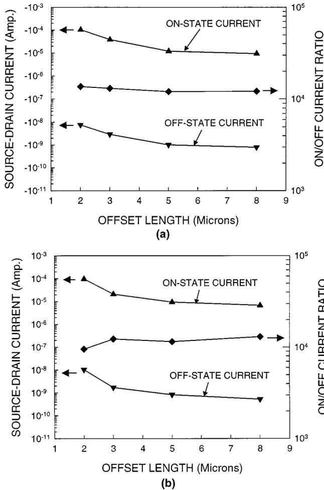
Fig. 6. On-state and off-state current versus offset length of the (a) p-channel poly-Si/Si<sub>1-x</sub>Ge<sub>x</sub>/Si CMTFT and (b) n-channel poly-Si/Si<sub>1-x</sub>Ge<sub>x</sub>/Si CMTFT.
