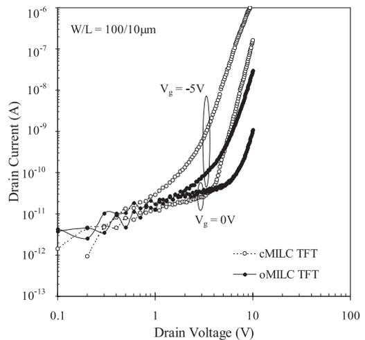
Fig. 4. Dependence of the leakage current of oMILC and cMILC TFTs on drain bias, at two different gate bias conditions.
