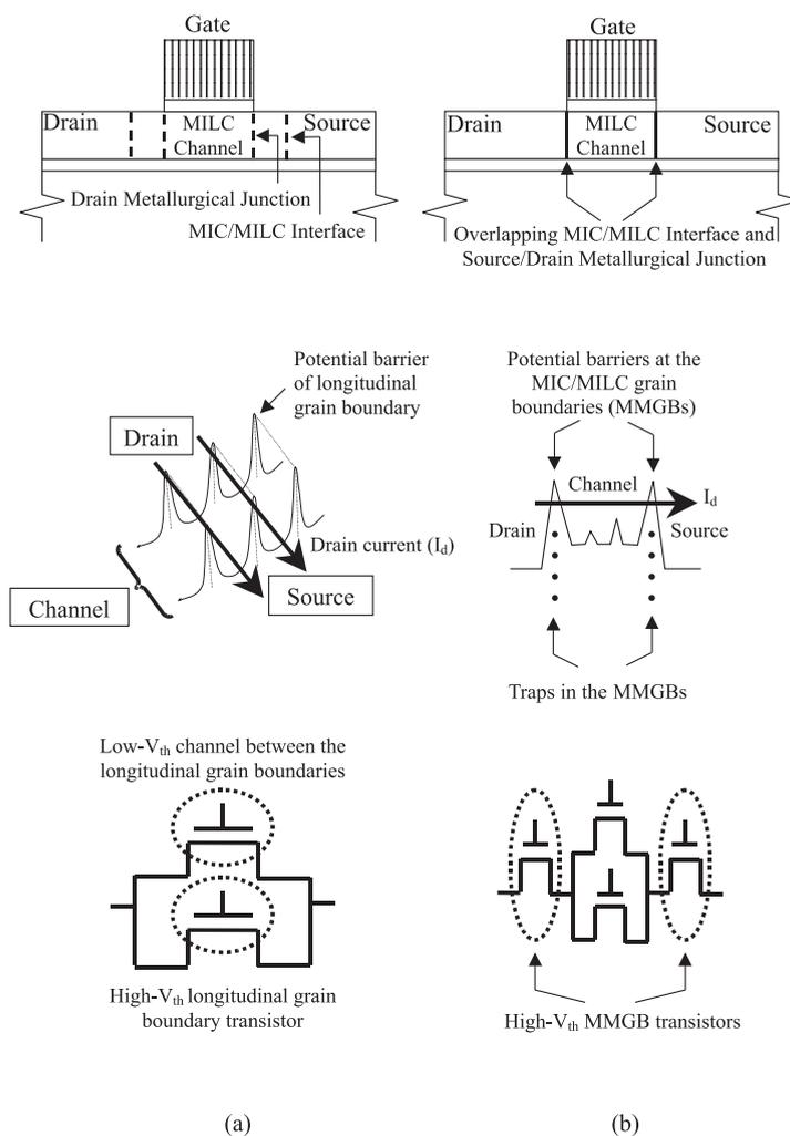
Fig. 1. Schematics of oMILC and cMILC TFTs. Also shown are grain boundary models and the low  $V_d$  transistor models of (a) oMILC TFT and (b) cMILC TFT.
