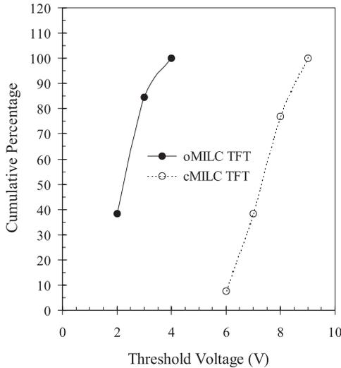
Fig. 3. Plot of cumulative % distribution of the threshold voltage of oMILC and cMILC TFTs.
