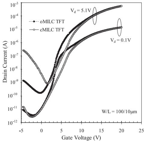
Fig. 2. Comparison of the transfer characteristics of oMILC and cMILC TFT.
