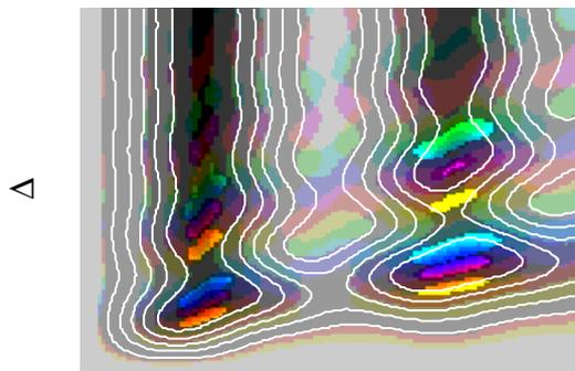
Fig.1 CPS diagram for transmissive LCD with  $\alpha=0^\circ$  and  $\gamma=0^\circ$
