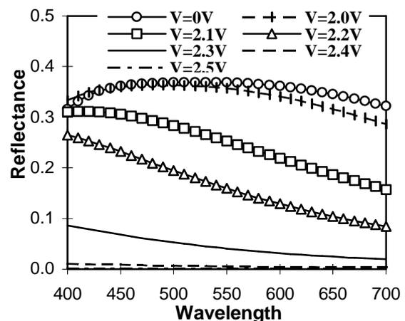
Fig.6 Simulation results of the output spectra of the fully compensated reflective STN cell under different voltages.
