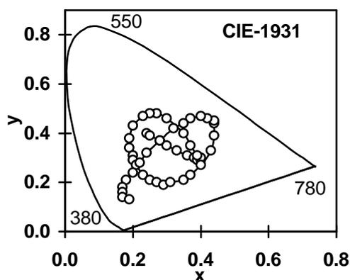
Fig.3 Experimental results of a multicolor STN cell in the CIE 1931 chromaticity diagram.
